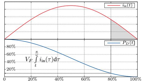
Figure 4. Diode losses
